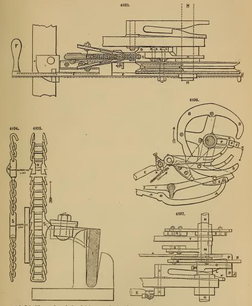
catch I is liberated, and the driving gut is thereby slackened and the machine stopped. Each plain link in the pitch-chain C represents therefore one row of loops or one course in the knitting, and each narrowing link represents a narrowing, and each stopping link represents the completion of the piece to be knitted.
